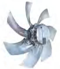
The air cooled condensers and dry coolers can be fitted with the new electronic fans developed using EC technology, dramatically reducing energy consumption. The fans are also fitted with a control system which can modulate the rotation speed depending on requirements, with excellent acoustic performance. The fans can be driven by a 0-10 Vdc signal or by BUS (RS 485).
